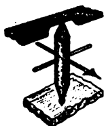
THE DOUBLE PIVOTED NEEDLE OF PEREGRINUS.
